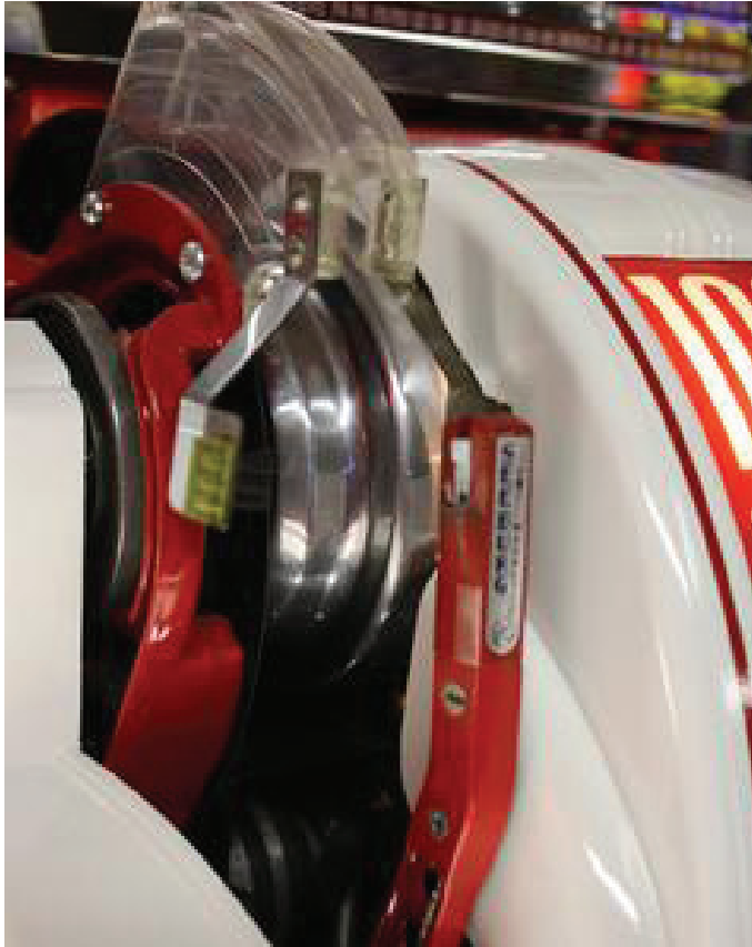
Records play vertically in the Seeburg M100B, which dates from 1954
